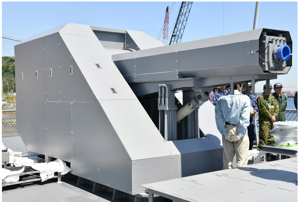
ABOVE: The rail gun on JS Asuka shown during inspection by the JMSDF Commander in Chief last month. Image: JMSDF
